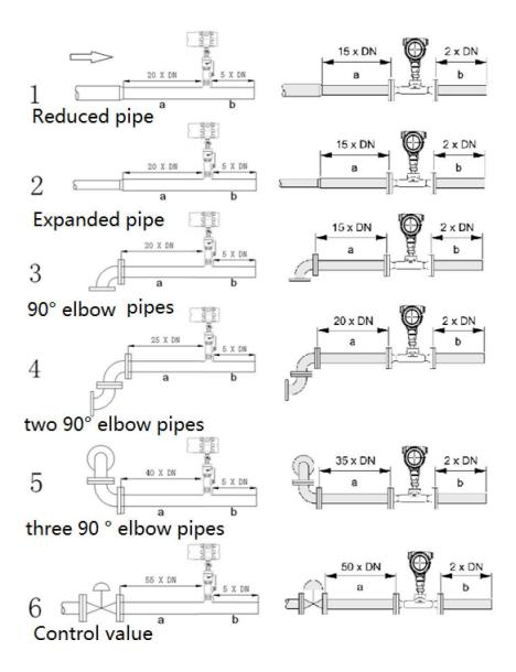
a = front straight section b = back straight section
