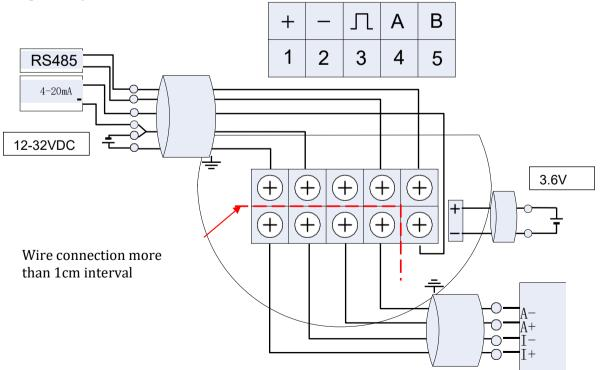
Battery-powered type uses H880BATDZ terminal wiring as follows:
