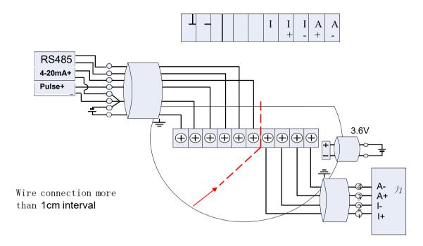
Instructions: Pulse wiring: +, -; ☐ Current wiring: +, -, I; RS485 wiring: +, -, A, B.
