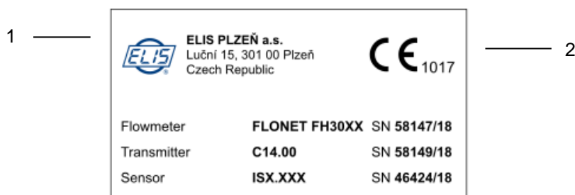
Example of the main meter plate
