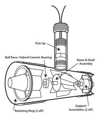
The Rotor and shaft assembly (1 off) which is mounted in ball race bearings, fitted inside Support assemblies (2 off) is turned by the kinectic energy of the flowing gas at an angular velocity, which in the linear range of the Flowmeter is proportional to the mean axial velocity of the gas.
