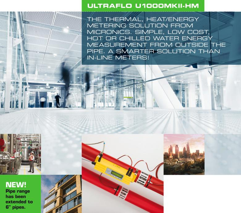
The U1000MKII-HM is an ultrasonic clamp-on thermal, heat/energy meter that uses ultrasound to measure flow rate and PT100 temperature sensors to measure flow and return temperatures. The U1000MKII-HM displays energy rate and totalised energy with pulse output and communication options, so it can be used as a standalone meter or as an integral part of an aM&T or BEM's system.
