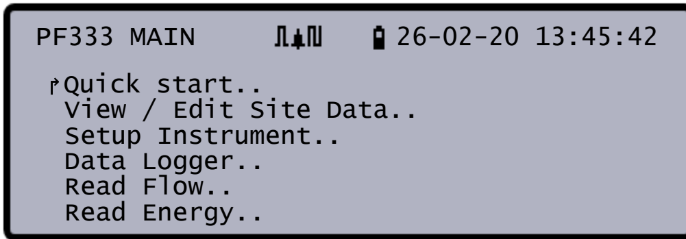
Figure 7 Main menu (Read Energy and Data Logger options available with PF333HM models only)
