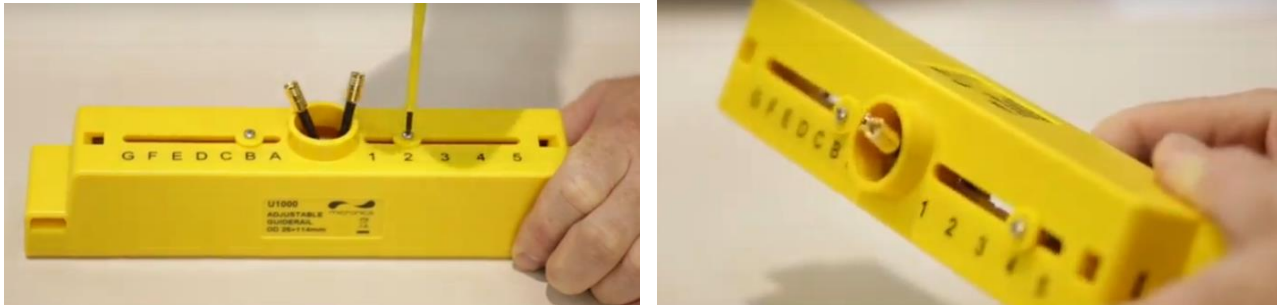
Figure 14 Loosen the flow sensor-holding screws (left); slide to correct position (right)
