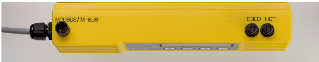
Figure 22 Temperature Sensor connectors on the Electronics Module
