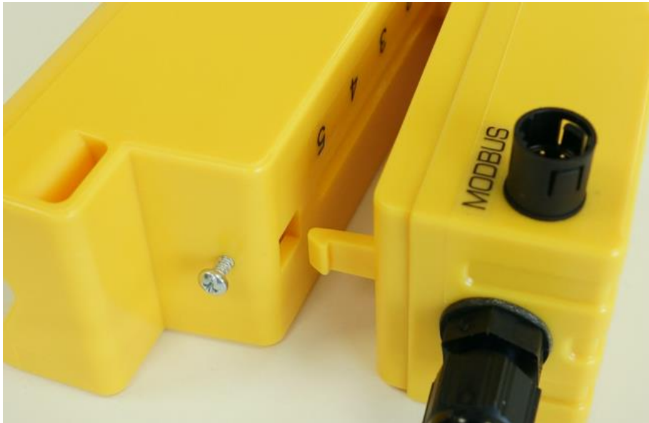
Figure 24 Separating Sensor Assembly and Electronics Module
