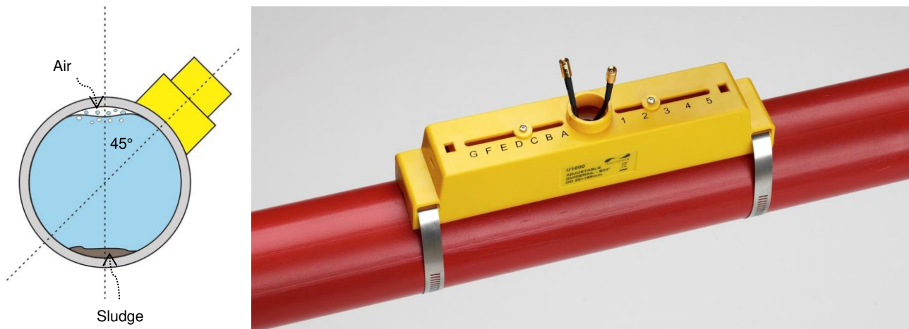
Figure 19 Sensor Assembly clamped at 45°
