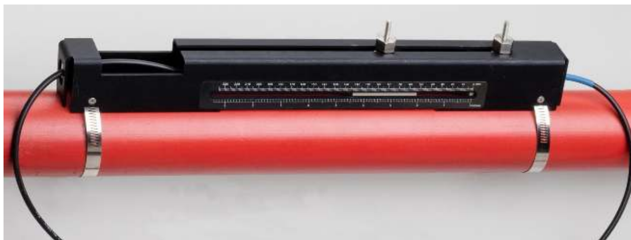
Figure 17 Lowering transducers onto pipe
