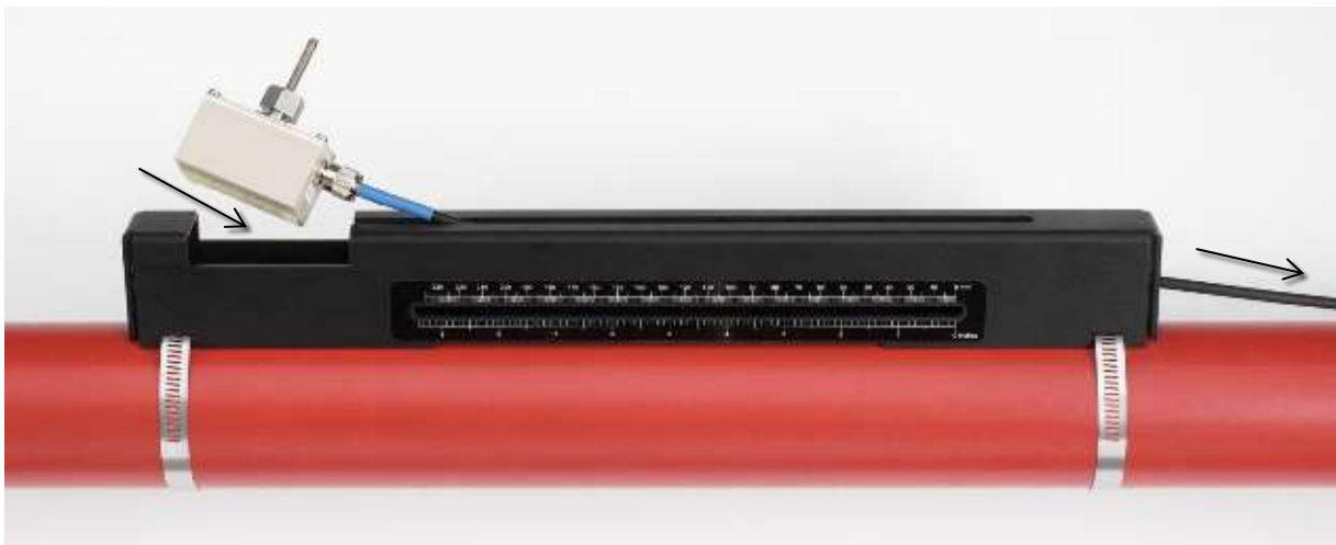
Figure 13 Installing downstream (blue) transducer
